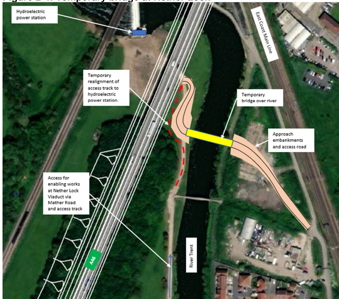
Figure 2-4: Temporary bridge at Nether Lock
